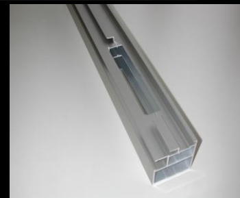
Tri-level removal of material from hollow workpiece
